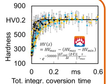
Fig.2 :PSK of the hardness-depth curve
